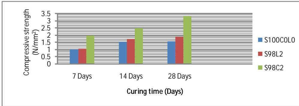
**Fig. 1:** Compressive strength of the control mix, 2% lime and cement stabilizations
