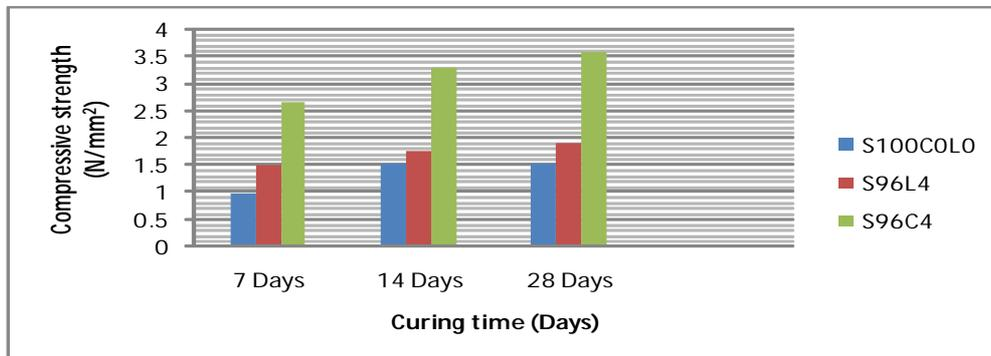
**Fig. 2:** Compressive strength of the control mix, 4% lime and cement stabilizations
