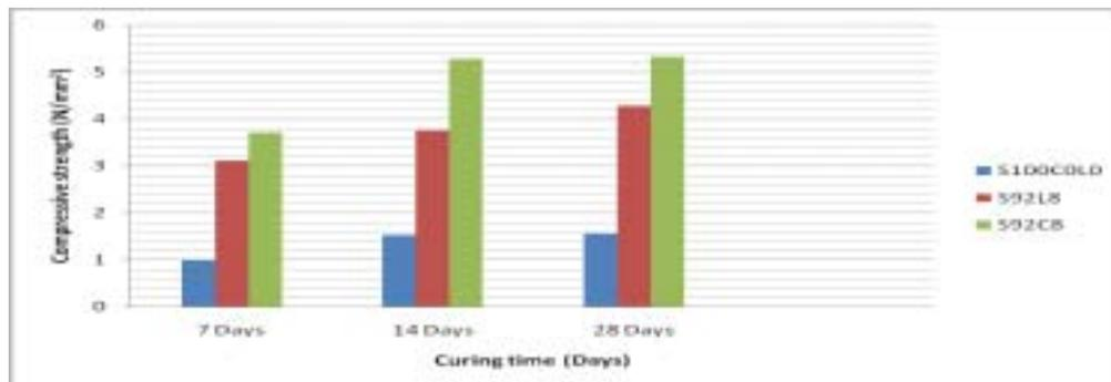
**Fig. 4:** Compressive strength of the control mix, 8% lime and cement stabilizations
