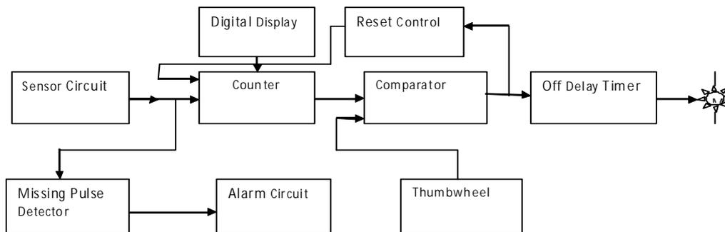
**Fig. 3:** Block diagram of an Automatic Control System of a Bottling plant
